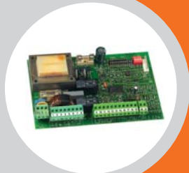
452 MPS control board
